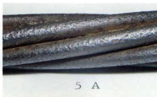
Photo 5A. Strand surface after cleaning.
