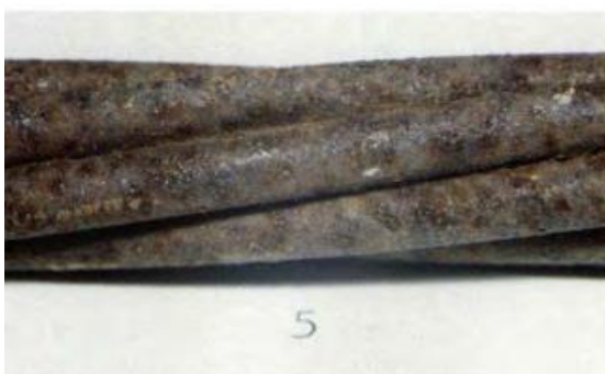
Photo 5. Strand surface before cleaning.
