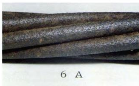
Photo 6A. Strand surface after cleaning.
