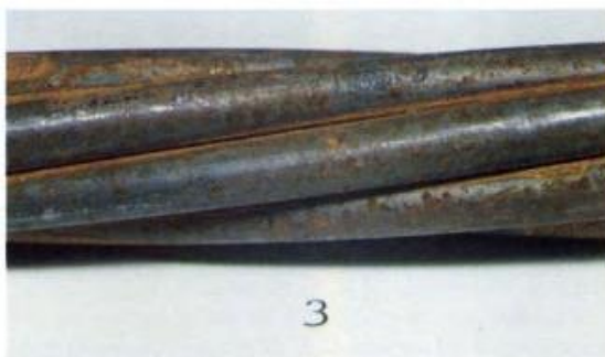
Photo 3. Strand surface before cleaning.
