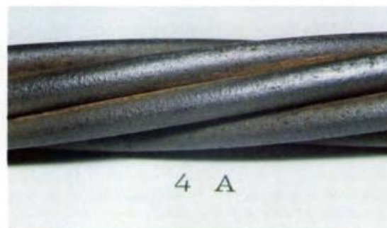
Photo 4A. Strand surface after cleaning.
