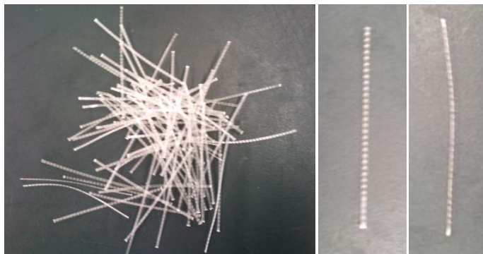
Fig.2.5 Macrofibra de polipropileno MasterFiber (MAC Matrix-BASF)
