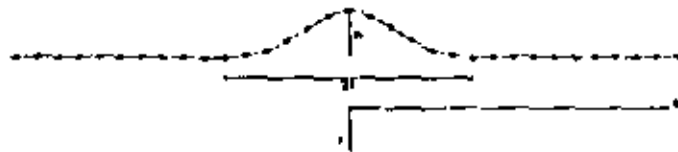
Figure 1. Geometrical shape of the mountain model introduced by Sills (1978), and corresponding to the cases investigated in Figs 2–17. The open circles indicate the sites where the synthetic seismograms of Figs 2, 3 and 14 are computed.
