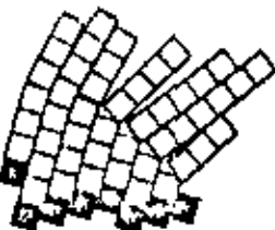
Computer produced drawings of toppling failure. After Cundall 20 . (Dark blocks are fixed.)
