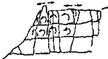
Suggested toppling failure mechanism of middle face of Yaourt slide. After Hofmann 26 and Moller 27 .
