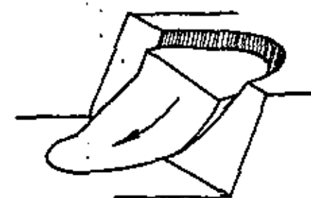
a. Circular failure in overburden soil, waste rock or heavily fractured rock with no identifiable structural pattern.
