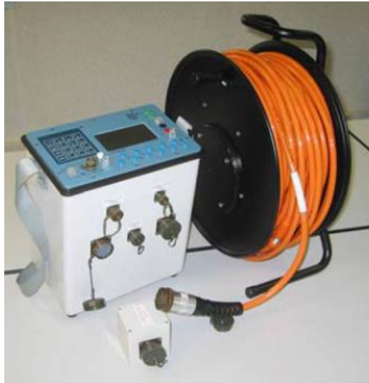
Figura 4.1.1 Consola SYSCAL PRO y cable multi-core .
