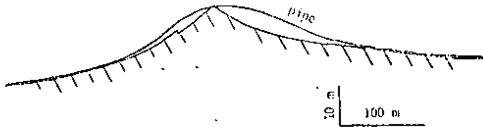
Figure 2: Section through sand wave (vertical exaggeration 5:1)
