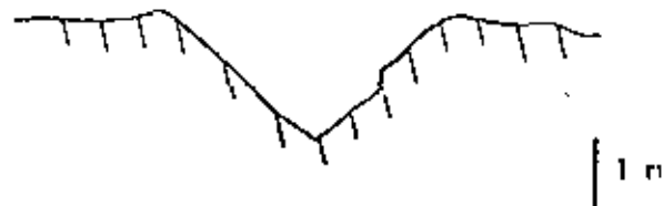
Figure 3: Trench section obtained by high frequency profiler
