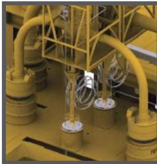
Figura 4.8 Pig loop del manifold.
