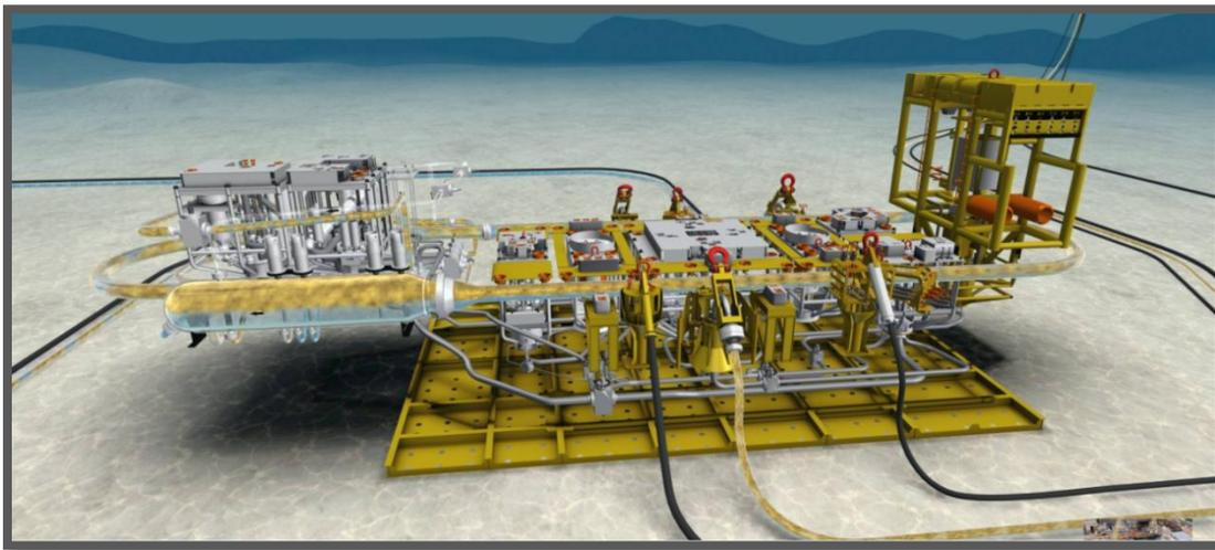
Figura 4.4 Manifold (FMC Technologies).
