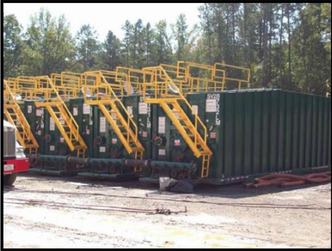
Figura 3.11 Contenedores de agua – Tanques “Frac” en la lutita de Fayetteville (Tomada de Evaluating Implications of Hydraulic Fracturing in Shale Gas Reservoirs, SPE 2009)
