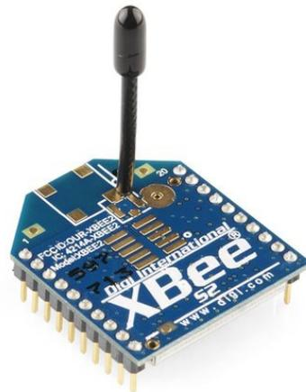
**Figura 21 Radio XBee Series 2.**
