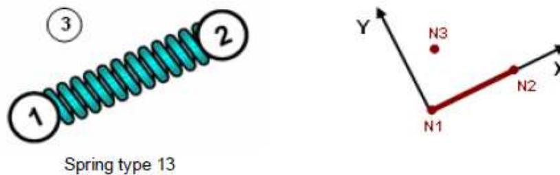
**Figura 4.5** Elemento *spring type 13 – beam* (Altair Engineering, *Radioss 11.0 User's Guide*, 2011).
