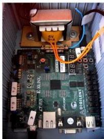
Figure 2. FPGA electronic controller for external hardware.
