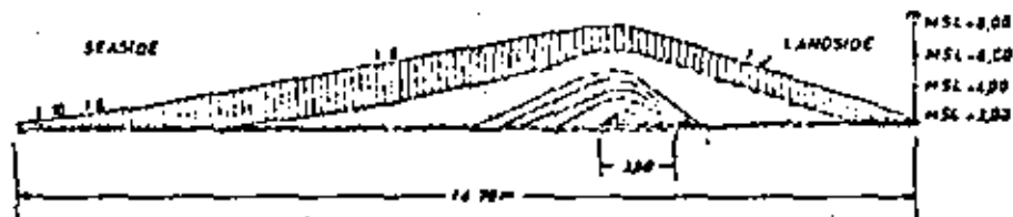
Fig. 21. Comparison of dikes with modern dune profiles (Frank, 1971)
