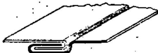
ACME OR GROOVED SEAM ALSO CALLED FLAT LOCK AND PIPE LOCK
