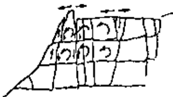
Suggested toppling failure mechanism of north face of Vajont slide. After Holmström and Müller 26 .
