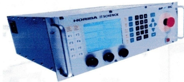
figure 20: manual control SPARC
