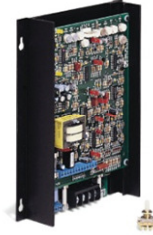
Fig. 3.3 Tarjeta de Control Baldor BC200
