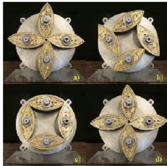
Fig. 2. Engine operating sequence. (a) start of admission, (b) near end of expansion, (c) exhaust in progress, (d) end of exhaust
