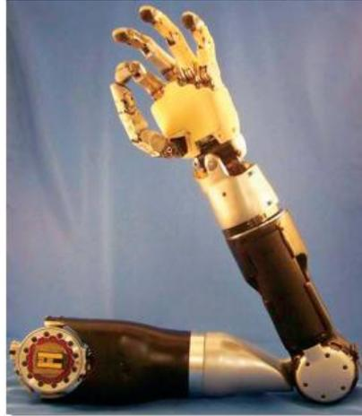
Fig. 1.12 Modular Prosthetic Limb [31]
