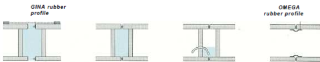
Figure 2.40 Conceptual processes for linking two elements (Trelleborg Baker, 2008)
