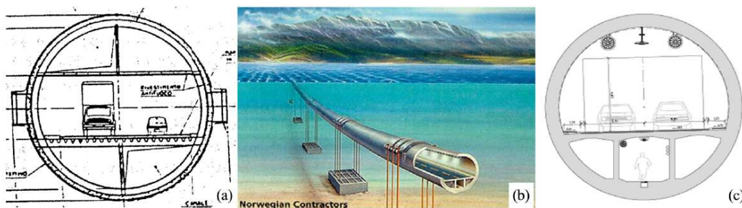
Figure 1.11 SFT with circular cross section. (a) Messina Strait crossing (Italy) proposed by ATI-SSST (Scolari et al., 1989); (b) Høgsfjord crossing (Norway) proposed by Aker Norwegian contractors (Skorpa and Østlid, 2001); (c) Sulafjord crossing (Norway) (Jakobsen et al., 2009)
