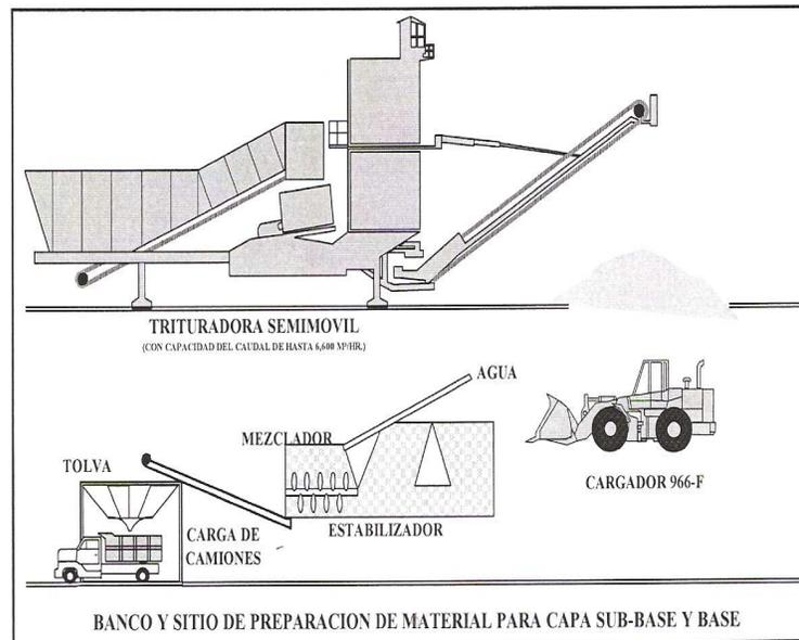
**FIGURA 2.4 "DESCRIPCION PARA OBTENER MATERIAL SUB-BASE Y BASE"**
