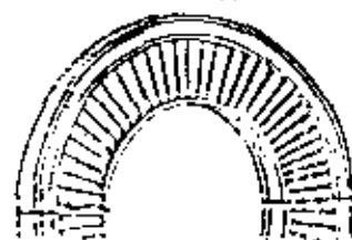
4 Typical nozzle setups are for disk-and-diaphragm unit, above; drum type, below
