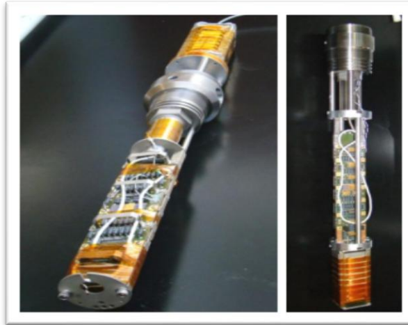
Figura 2.15 Sensor de fondo Pan American Energy.
