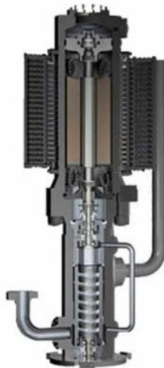
FUENTE: FMC Technologies FIGURA 4.18, "BOMBA SUBMARINA HELICO-AXIAL"
