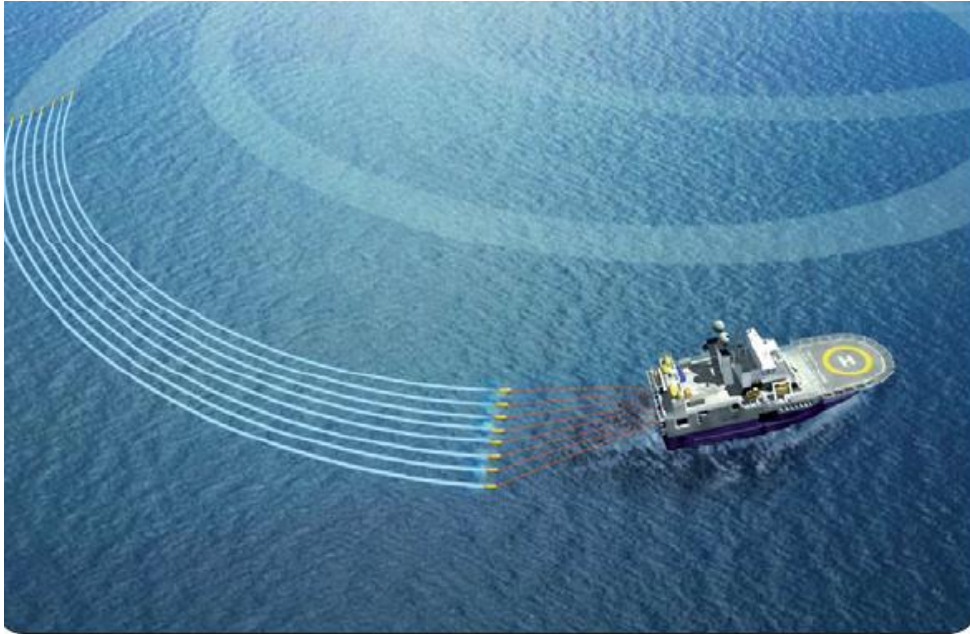
FUENTE: New seismic technologies for deepwater succes FIGURA 1.2, "TECNOLOGÍA COIL-SHOOTING"
