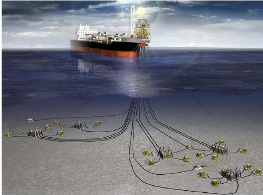
FUENTE: Subsea structural engineering FIGURA 4.27, "TIE-BACK SUBMARINO A FPSO"
