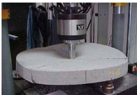
**Figura 1.15** Ensayo de panel circular (ASTM C1550)
