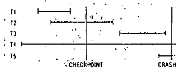
Figure 7. Five transaction types with respect to the most recent checkpoint and the crash point. At restart, T2 and T3 will be redone while T4 and T5 will be undone. Since T1 ended before the checkpoint, its outputs already appear in the checkpoint.
