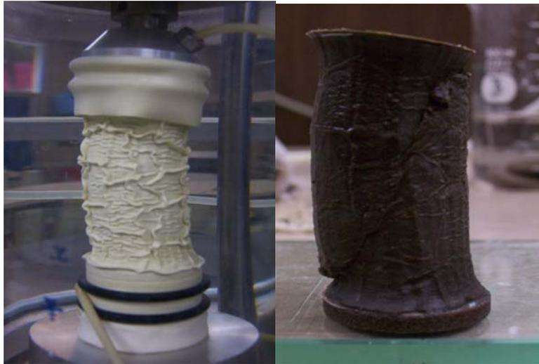
Foto 5.1. Probeta OCR = 1, 0.1 %/h
