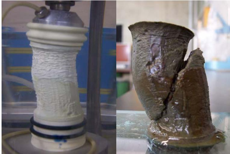
Foto 5.5. Probeta OCR = 3, 0.1 %/h
