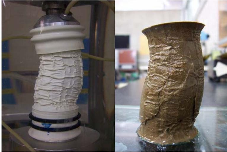
Foto 5.13. Probeta OCR = 8, 0.1 %/h
