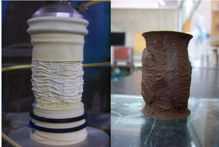
Foto 5.17. Probeta OCR = 11.8, 0.1 %/h
