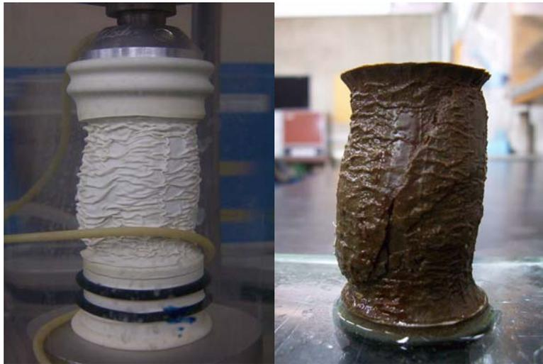
Foto 5.9. Probeta OCR = 6, 0.1 %/h
