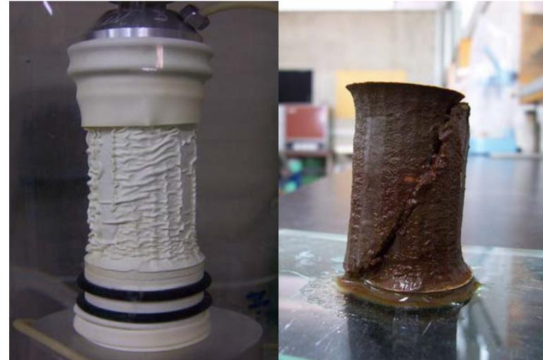
Foto 5.20. Probeta OCR = 11.8, 100 %/h
