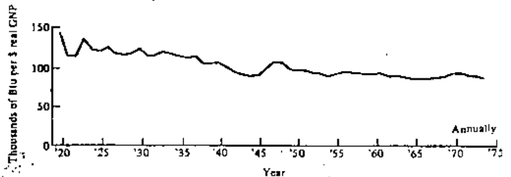
Fig. 1.6 Energy consumed per unit of economic output (real GNP in 1958 dollars) in the U.S.A.
