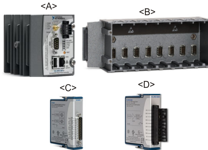
Figura A.3: Sistema cRIO, (A)NI-9014, (B) NI-9004, (C)Ni-9401, (D)NI-9263.
