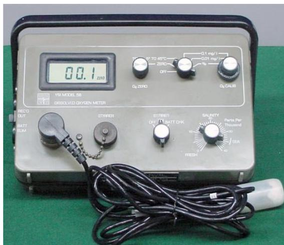
Figura 5.12. Dissolved Oxygen Meter YSI Model 58
