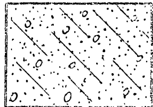
RELLENO DE MATERIAL PERMEABLE
