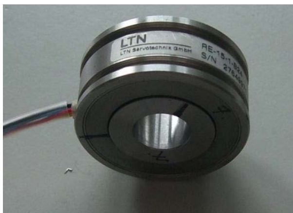
Figura 4-67: Encoder LTN Servotechnik RE 15-1
