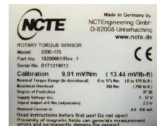
$V_{out(max)}$  and  $V_{out(min)}$  are defined with the slope of the sensor. i.e. the output voltage could be between 0.5V and 4.5V. The actual signal output range depends however on the calibration value.
