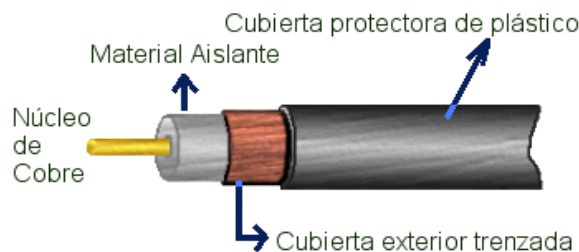
Figura 3.5 Cable coaxial
