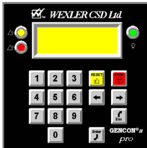
Figura 4.12 Control GENCON II Vista Frontal
