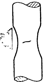
FIG. 15.2. Longitudinal sections of a tensile specimen of mild steel just prior to fracture, showing the development of an internal ductile fracture crack starting at the center of the necked-down portion of the tensile specimen.
