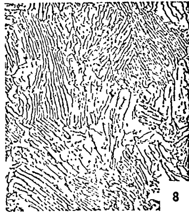
Micro. 8.7. 0.8% C + 0.65% Mn steel, annealed by furnace cooling from 810°C;
