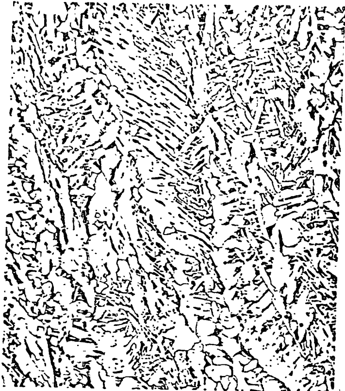
FIG. 21.9 Structure of deposited metal zone in welded steel (250x).
