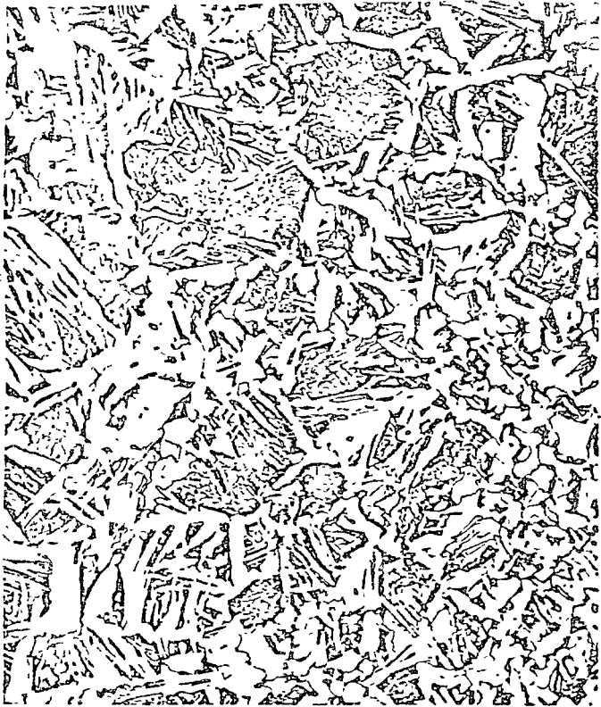
FIG. 21.7 Structure of coarsened zone in welded steel (250X).
