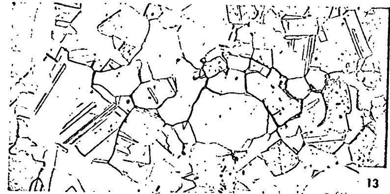
MICRO. 4.13. Annealed 70-30 brass subjected to a tensile stress of 10,000 psi in
