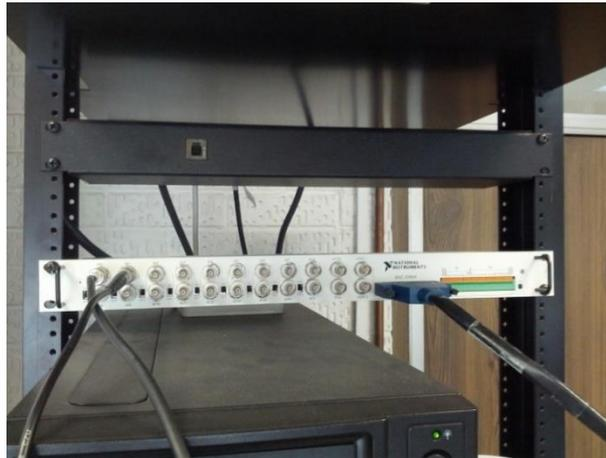
**Figura 85. Multiconector BNC-2090A**
