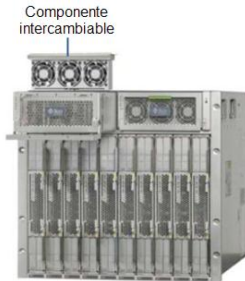
Figura No.4.4-Chassis Sun Blade 6000, componente intercambiable.
