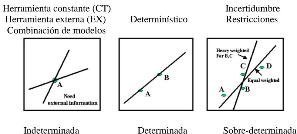
Figura 58. Soluciones dadas por ELAN, (tomada de ELANPlus GeoFrame Advanced Petrophysical Interpretation, Schlumberger Information Solutions, 2003).
