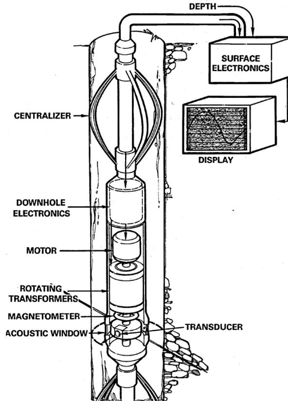
Fig. 50. Registro borehole televiewer (BHTV). (Steingrímsson, 2011).
