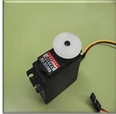
**Figura 2.6 Servomotor**
