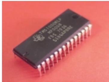
Figura 2.2. Microcontrolador Texas Instruments TMS1000.
