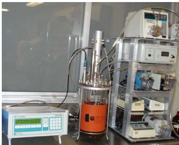
Figura 4.4 Reactor anaerobio SBR
