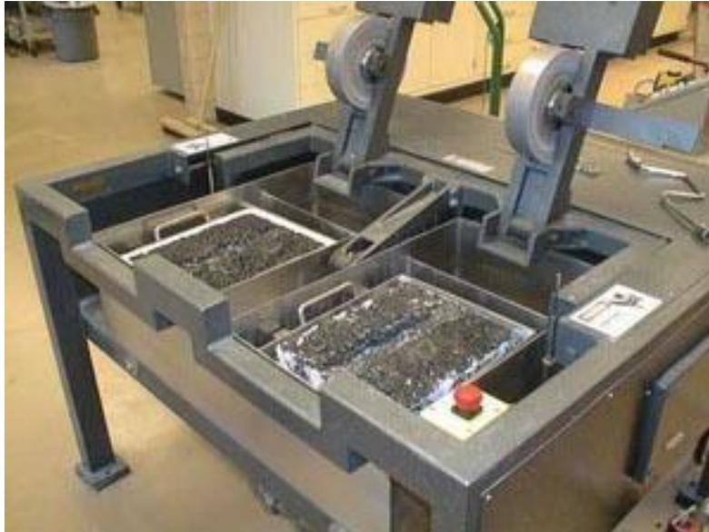
**Rueda de Hamburgo.** Fuente: <http://www.fhwa.dot.gov/pavement/asphalt/labs/mixtures/hamburg.cfm>
