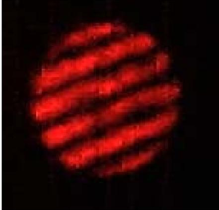
Fig. 8. Interferometric pattern, obtained with wavefronts with an intersection angle major of 10 degree.
