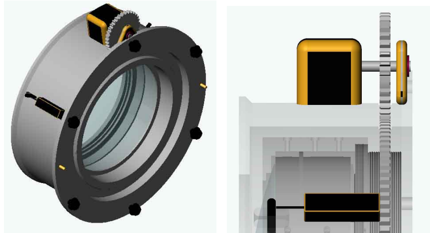
Figure 4.7 First barrel stage (barrel#1) with the B1C1 cell and the Focusing Unit. Bolts fix the barrel to the interface with the shutter and the supporting structure of OSIRIS
