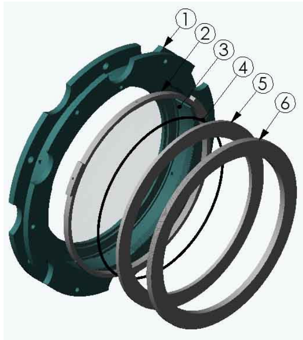
Figure 4.6 The B2C2 cell, holding singlet S1, as an example of cell components. Shown are (1) the cell, (2) the Radial Support ring (RSS1), (3) the lens (S1), (4) an O-ring and (5, 6) the separators. All other lens cells in the OSIRIS CB have the same concept and components.
