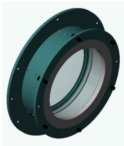
Figure 4.8 The B2C1 cell holding doublet lens D2: assembled view, elements as in Figure 4.6. The face with larger radius connects to the OSIRIS shutter and support interface.
