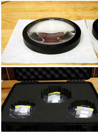
Fig. 11 Image of lens S1 with coatings in its container for protection. The bottom image is the transportation briefcase for three of the eight lenses.
