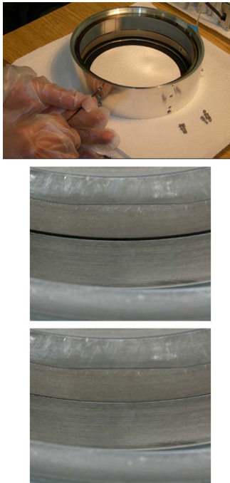
Fig. 13 Deformation achieved due to traction force of the screws; before and after.
