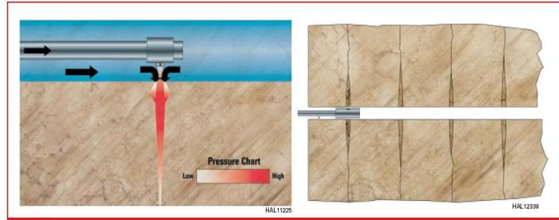
Fig. 6 - In the SurgiFrac process, sand-laden fluid pumped through a Hydra-Jet™ tool impinges on the formation creating a cavity. As the cavity is formed, pressure on the bottom of the cavity increases, eventually initiating a fracture. Annular fluid is pulled into the fracture, helping to extend it.
