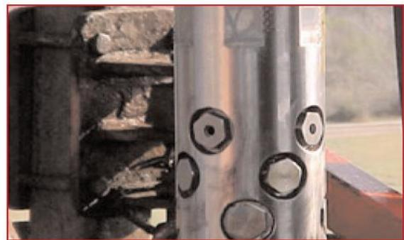
*Fig. 8 – SurgiFrac<sup>SM</sup> service uses a specially designed high-pressure hydrjetting tool similar to those commonly used in oilfield applications to abrade, penetrate, or cut steel casings or rock formations. The tool can be designed to meet well conditions.*
