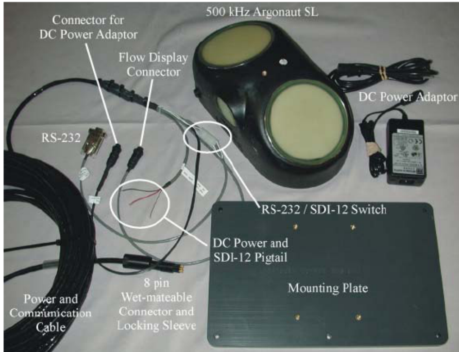
Figure 5-13. 500-kHz Argonaut-SL with Standard Equipment
