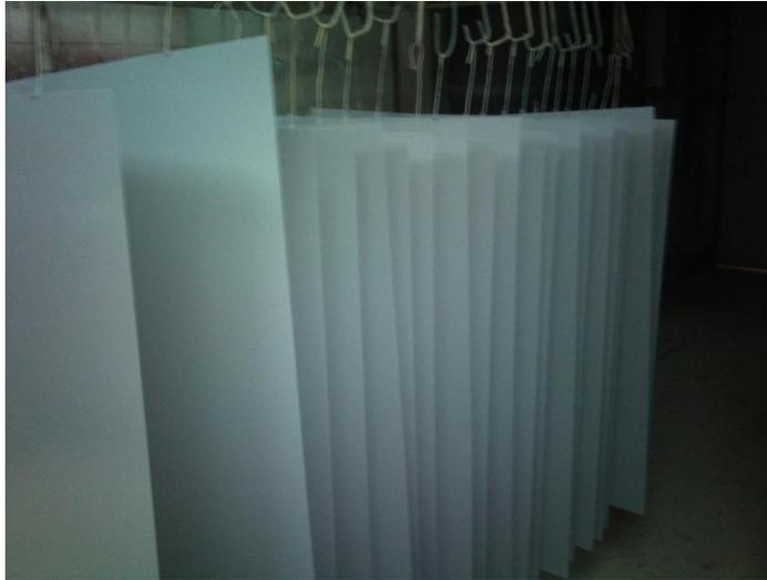
**IMAGEN 6.6. CONJUNTO O LOTE DE LÁMINAS CON PINTURA ELECTROSTÁTICA, LISTAS PARA SER HORNEDAS**
