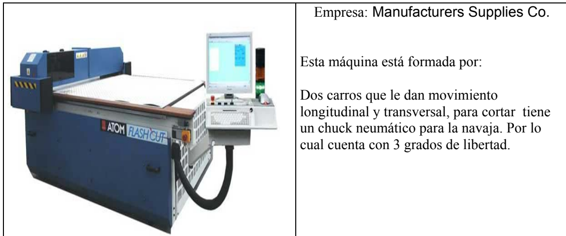
Figura 1.9 Modelo: ATOM Flashcut Model 15155 Oscillating Knife Cutting System.
