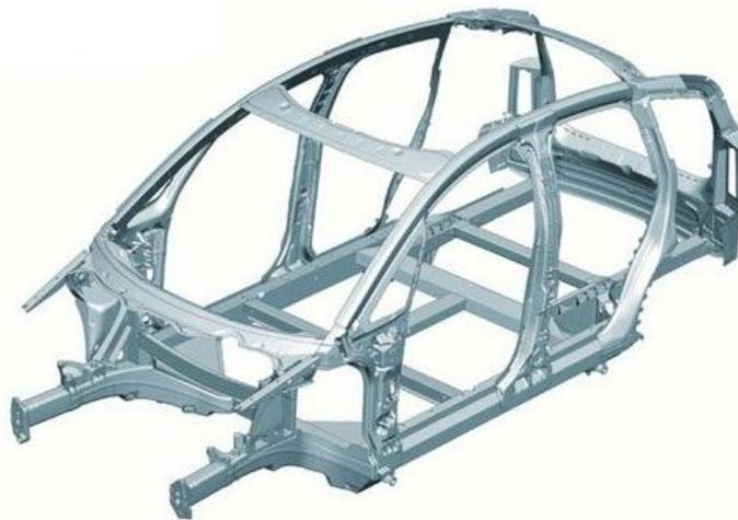
FIGURA 1.7 ESTRUCTURA DE UN AUDI A2 EN ALUMINIO [8]
