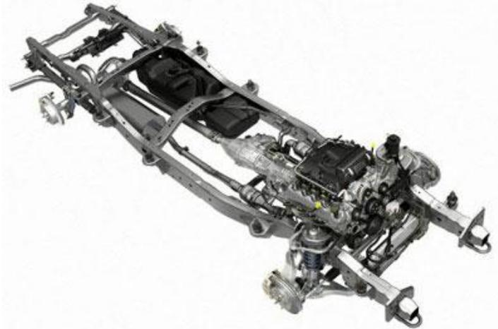
FIGURA 1.3 BASTIDOR MONTADO (CHASIS INDEPENDIENTE) [3]
