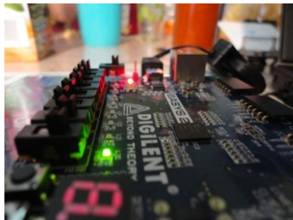
Figura 3.3.19 SW0: alto SW1: alto LD0: alto
